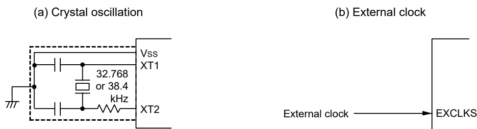
Figure 6-21. Example of External Circuit of XT1 Oscillator
